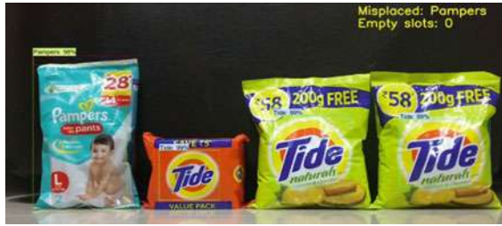
Fig. 10 Misplaced object identification, but no shelf space
