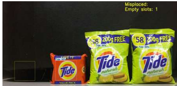
Fig. 8 Empty slots detection and real-time update
