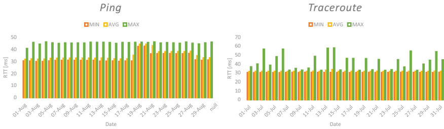
Fig. 1 Ping (left) versus Traceroute (right) day-to-day minimum, average, and maximum RTTs for Denmark ('north→south' direction)
